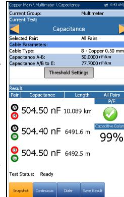
**Note:** The accuracy of the **2 Terminal Capacitance Measurement** is impacted by the use of the **FED**, and the **3 Terminal (default) method** is recommended to be used instead.
