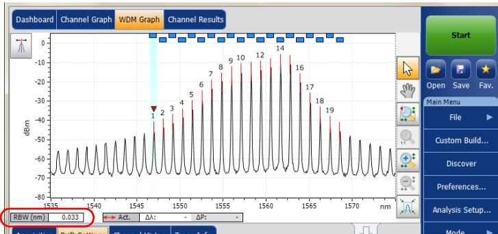
The graph will display peak indicators for all the channels found by the application with a red vertical line over the peaks to indicate the peak position.
