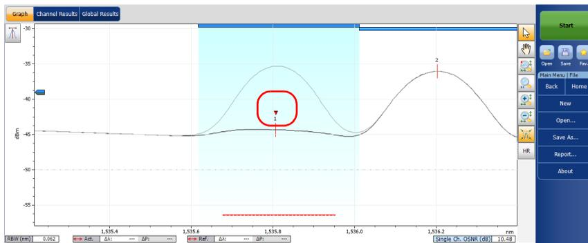
The noise level for a channel is indicated by a dotted line under the selected peak. The width of the noise level indicator is set according to the current Noise for OSNR setting. The width of the noise level indicator depends on the noise associated with the OSNR setting (from the largest to the narrowest): IEC, InB, InB nf, Pol-Mux and fit.
