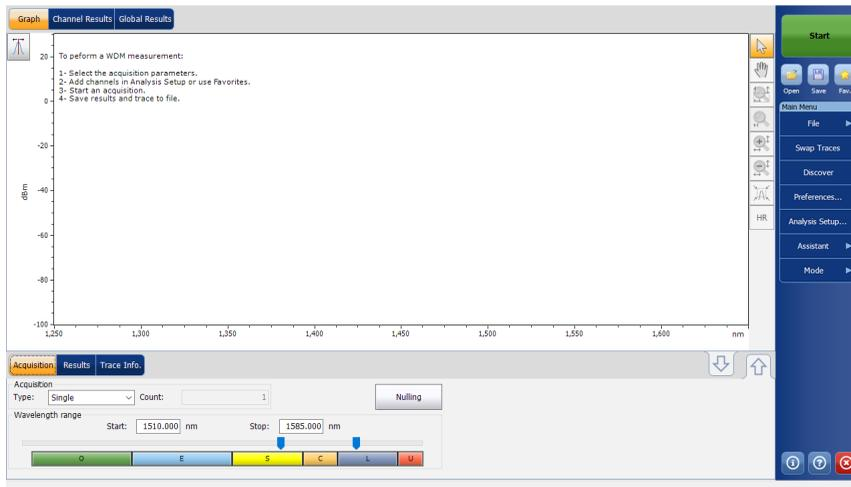
When the acquisition is taken (see *Starting a Measurement* on page 249 for details on how to perform a test), the active trace will be displayed in the tab with information along the following axis values:
