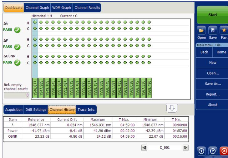
You can select a channel directly from the dashboard or from the **Channel History** tab. For each channel, the dashboard displays the pass/fail status for each of the following parameters:
