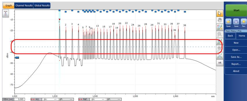
A peak detection level cursor is available in the graph when the **Results** tab is selected. The cursor is positioned along the Y-axis in accordance with the application's peak detection level global analysis parameter.
