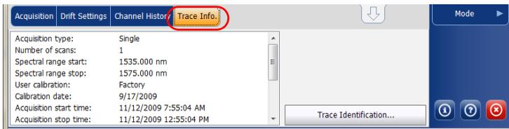
2. For some test types (WDM if there is a reference trace, spectral transmittance and EDFA), select which trace you want to view.
