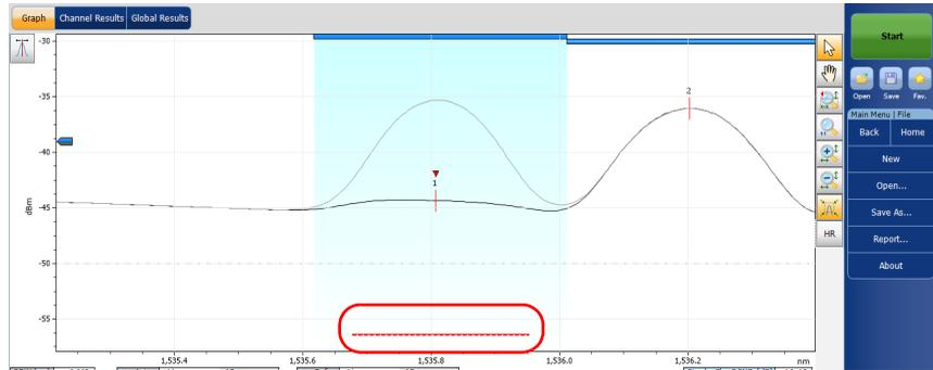
A dotted line across the full spectral width corresponds to the peak detection level indicator. This line indicates the minimum power level (dBm) from where a peak can be considered as a valid signal.
