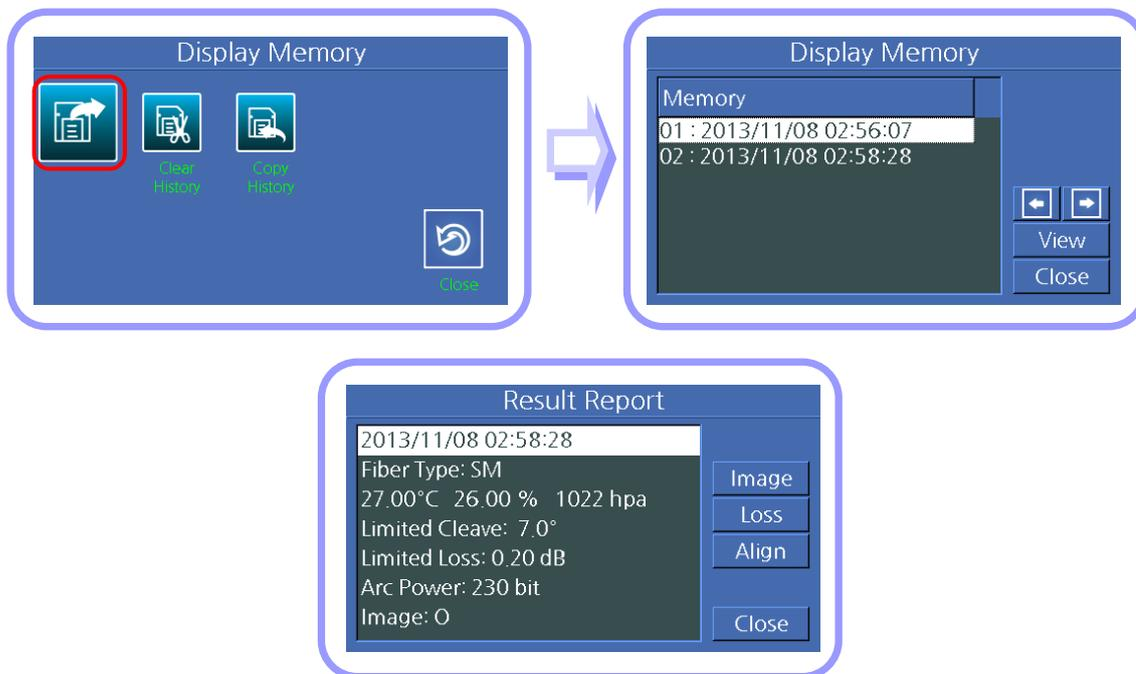
Image : This is shown only if image capture is executed after splicing.
