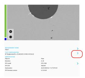
**2.** To enter the edition mode, press and hold any test configuration in the **Test Configuration** window.
