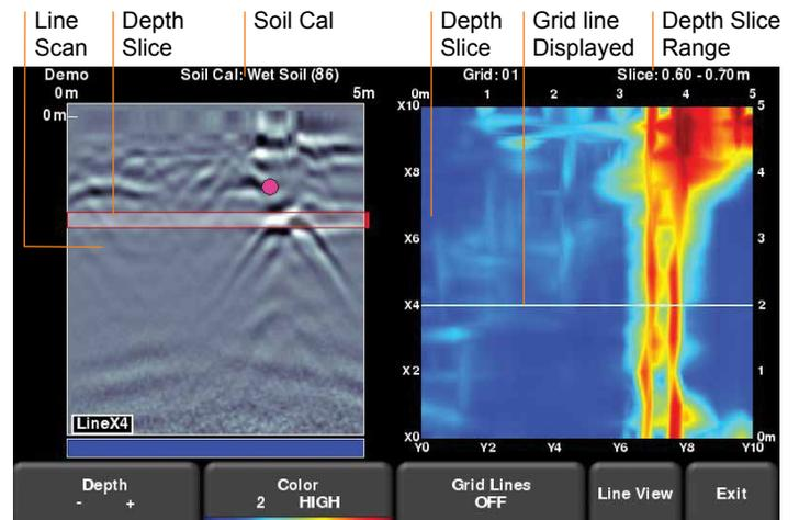
Pressing the + and - buttons on the **Depth** button will increase or decrease the depth of the depth slice currently displayed. This allows the user to "slice through" the ground, and locate features that appear at different depths.
