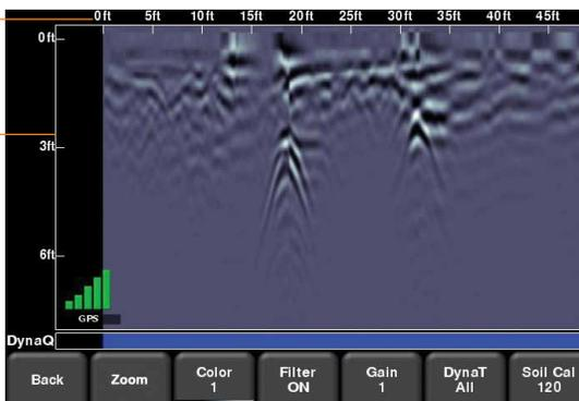
To locate targets, move the system back along the same path until the red vertical line is exactly over the response (usually a hyperbola). You can mark the location of the object on the surface and continue data collection. Viewing options can be adjusted using the menu at the bottom of the screen.
